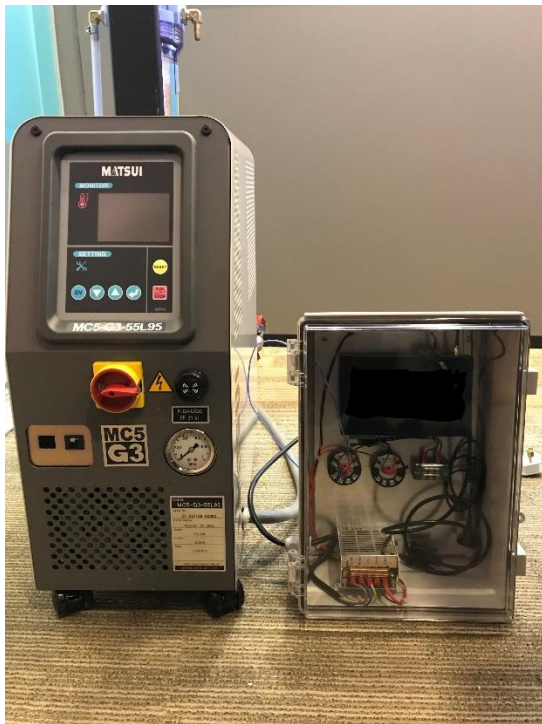
Mobile-connected mold-temperature controller system
